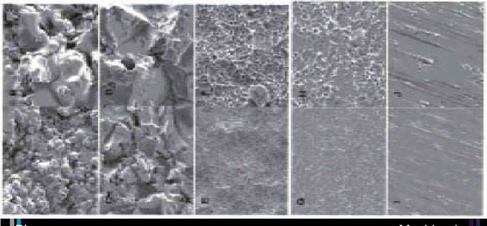
PlasmaGrit-blastedGrit-blastedDual acid-Machinedsprayedand dualetched(turned)(TPS);acid-etchedDavies, 2003
