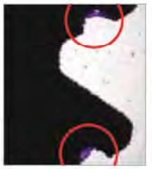
FROOW BONE FORMATION Faster bone growth within the groove results in enhanced rate of osseointegration and biomechanical stability.
